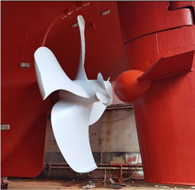
CLT propeller with advanced PBCF
